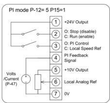
Remote closed loop PI feedback control with Local Analog speed input
