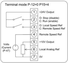
Local or remote analog speeds (2 analog inputs)
