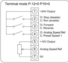
Analog speed input with 1 preset speed and fwd/rev switch
