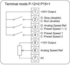
Analog speed input with 2 preset speeds
