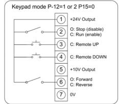
Remote push button speed control with fwd/rev
