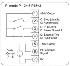
Remote closed loop PI feedback control with Local Preset speed 1 and motor thermistor trip
