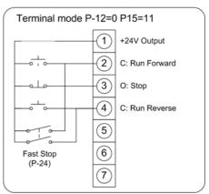
Push button fwd/rev/stop with fast stop using 2<sup>nd</sup> deceleration ramp
